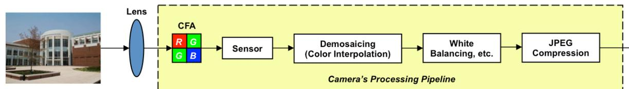
Figure 1: A typical digital camera's internal processing pipeline.
