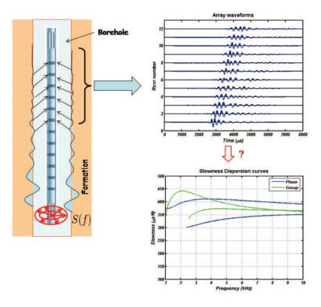
Fig. 1. Schematic showing the generation and acquisition of acoustic waves by the sonic tool in a fluid filled borehole on the left. The corresponding dispersion extraction problem consists in using the array waveform traces collected at one depth as shown on the top right to estimate the dispersion curves shown on the bottom right.
