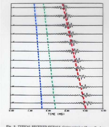
Fig. 2. TYPICAL RECEIVED SIGNALS. Casing arrival at 57  $\mu$ sec/ft. dominates the early part of the waveform. Formation compressional slowness = 70  $\mu$ sec/ft., shear slowness = 138  $\mu$ sec/ft, sampling rate = 100 kHz, spatial separation = 6 inches.
