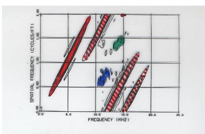
Fig. 4. CONTOUR PLOT OF FOURIER SPECTRUM. Only frequencies from 0 to 25 kHz are shown since the effective bandwidth of the signals is about 20 kHz.
