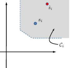
Quantization ZF precoder  $\mathcal{Q}(\mathbf{Ps}) = \mathcal{Q}(\mathbf{H}(\mathbf{H}^T\mathbf{H})^{-1}\mathbf{s})$  eliminates scaling due to  $(\mathbf{H}^T\mathbf{H})^{-1} \to \beta \mathbf{I}$  scaling which "props up" weak channels and scales down strong channels in order to enforce  $\mathbf{s} \simeq \mathbf{H}^T\mathbf{x}$ .
