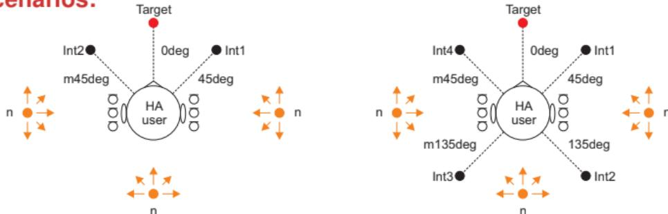
$d_{\text{mic}} = 15\text{cm}$ , source-mic dist.  $1.1\text{m}$ ,  $T_{60} \approx 300 \text{ msec}$ ,  $\mathbf{S}_{nn}(\omega)$  known!
