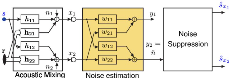
**Idea: Extend ICA-BSS cost function by geometric constraint** suppressing signals with target TDOA  $\tau_s$  ('null steering'):
