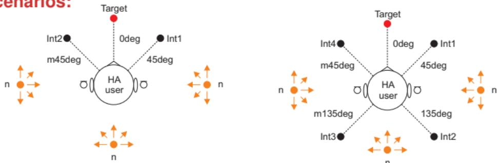
$d_{\text{mic}} = 15\text{cm}$ , Source distance 1.1m,  $T_{60} \approx 300 \text{ msec}$ ,  $f_s = 16\text{kHz}$
